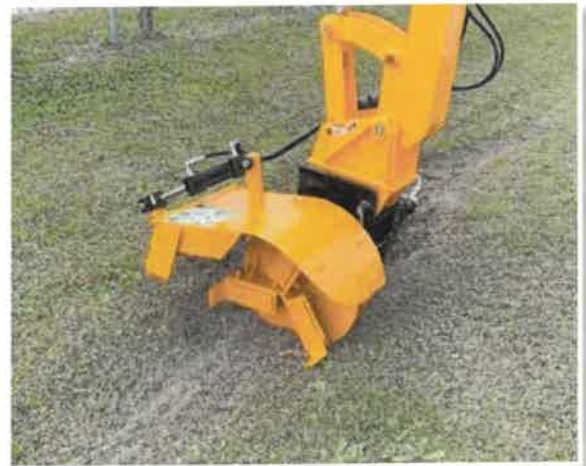
22in Ditch Maintainer with Adjustable Hydraulic Chute
