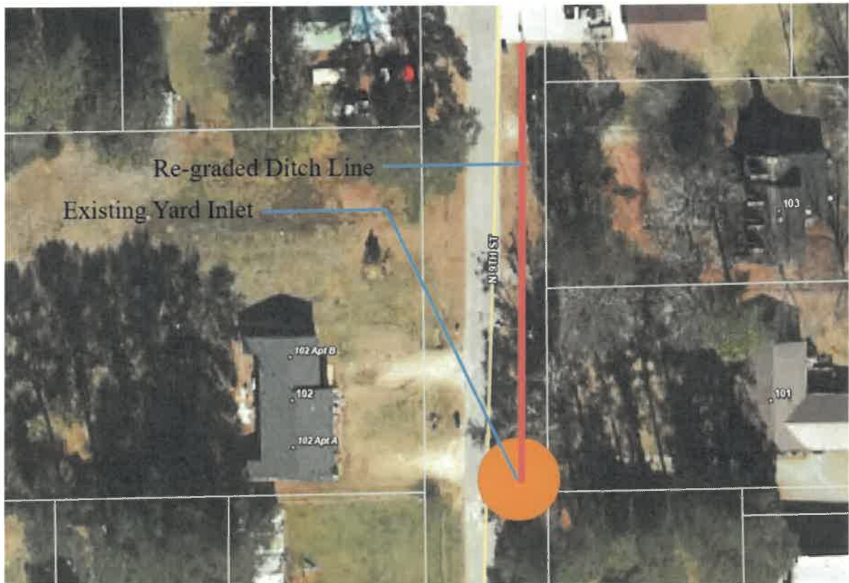
Project area showing ditch line to be re-graded and the location of the existing yard inlet.
